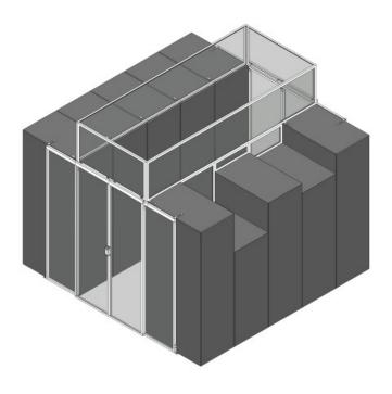
Rigid Containment is built with an aluminum frame and either clear or corrugated panels. Used in both hot and cold aisle containment, the panels can be made to fit the gaps created from inconsistent cabinet heights, obstructions, and spaces between cabinets and ceiling. The panels are shipped assembled and with hardware for easy installation.
